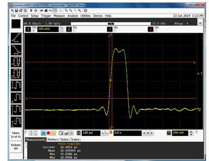
Figure 5. 100 ps pulse with 17 ps risetime.
